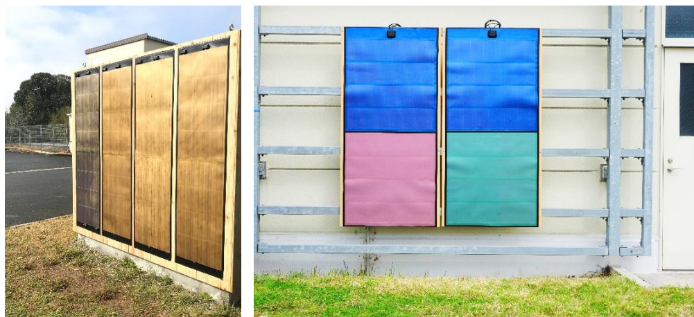
The verification tests feature flexible photovoltaic modules with wood-grain pattern decorative films (left) and monochrome decorative films (right) in actual-use environments
