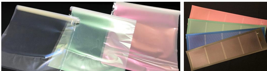
Decorative films before (left) and after (right) being applied to photovoltaic modules
